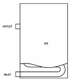
Extremely Thin Ice Formation at Evaporator Inlet
